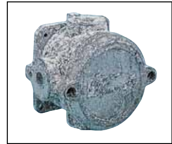
CORROSION ON A NON-TREATED PRODUCT.
