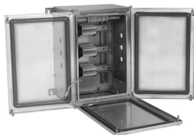
Reversible door. Opens to 210°, top, bottom, left or right, by moving the location of the hinges
