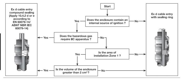
Note: Cable must be substantially compact and circular with an extruding bedding, and if any filters are used they are Non-Hygroscopic.
